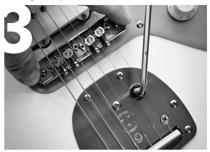
**With** the medium size Allen wrench, tighten the mounting post screws. (Do not over tighten!)
