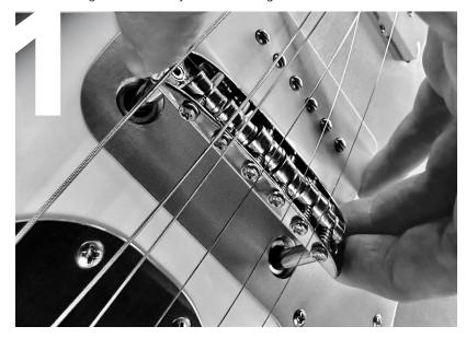
**Using** the medium size Allen wrench, slightly loosen the mounting post screws.
