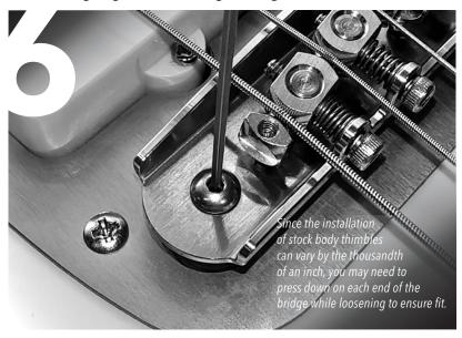
**Tune** instrument to pitch. Fine-tune the action with the four saddle height screws. To adjust the intonation after installment, use the large Allen wrench.
