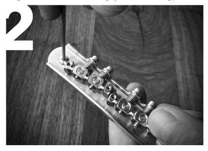
**Insert** bridge into body thimbles and press down on each end to ensure fit.
